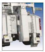
Full Hydraulic Independently Operated Rear Stabilizers Include Recovery Anchors
