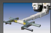
Adjustable Bus Arm Grids Quickly Attach for Wheel Lifting
