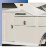
Lightweight, Corrosion-Proof, Bonded Composite & Aluminum Body
